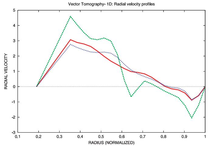
Fig. 6. Radial velocity profiles (dimensionless) at three different time moments: 180 \mu\text{s} (green), 193 \mu\text{s} (red) and 200 \mu\text{s} (blue).
